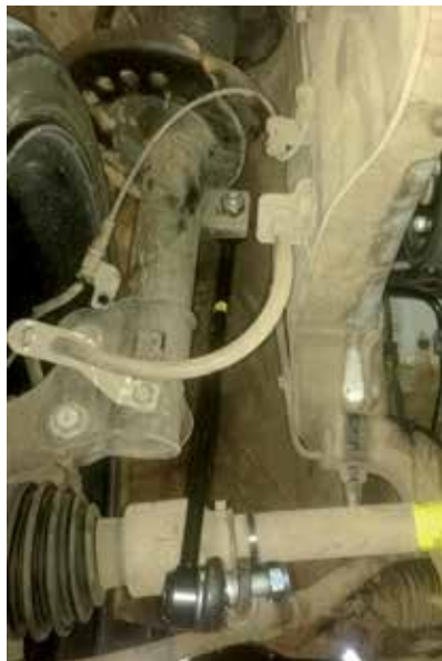
A bieleta nova instalada no Sonata
