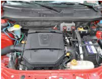
O motor E.torQ 1.6 Flex gera 117 cv
